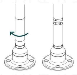
8. With the aid of the Allen key number 4, loosen the 3 internal screws on the side.
