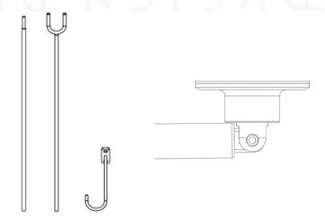
You will receive your pole with the joint locked, so if you want to use it as an articulated bar, you will first need to loosen the through screw that is mounted at the bottom of the upper base and also screw the hook and the upper base to the ceiling.
