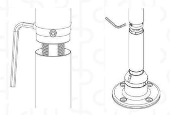
**15.** Raise and screw the protective cap counterclockwise until it is completely closed. It is not necessary to press it.
