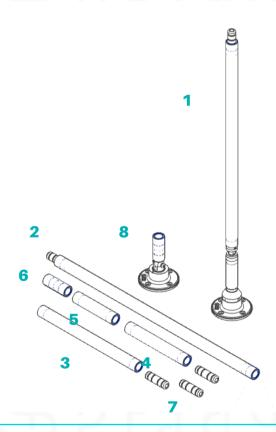
Atention: Parts are lubricated with Vaseline to facilitate fitting and removal.
