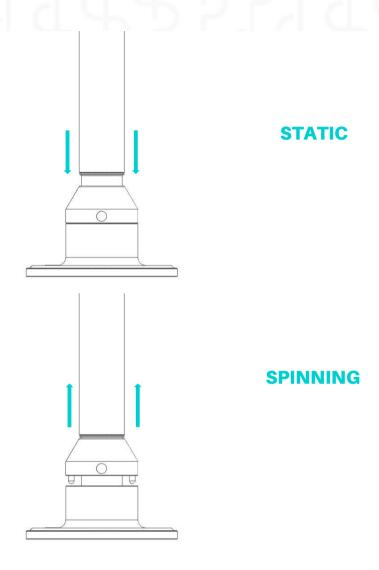
If your pole is not rotating homogeneously, that is, it creates a spring effect or resistance to rotation at a certain point, this is an indicator that it is not perfectly vertical or that the floor and ceilings may not be parallel.
