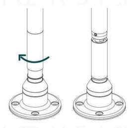
**8.** With the aid of the Allen key number 4, loosen the 3 internal screws on the side.
