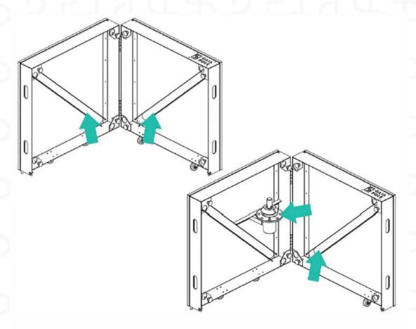
5. Now, open the case fully and rest it on the floor. Do this same procedure with both and fit one half on the other.
