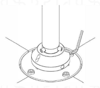
9. Fit the middle bar and tighten the side screw.
