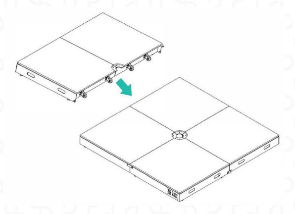
6. Fit the housing bearing in the center of the stage and with the aid of the Allen key number 6, insert all the 4 (four) screws.
