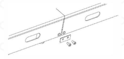
8. Fit the lower bar to the housing bearing and tighten the 3 side screws using the Allen key number 4.
